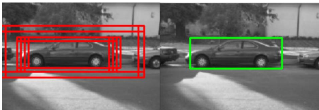
Figure 16: non maximum suppression (NMS). Overlapping boxes are being suppressed so only one box (with the highest confidence) survives
